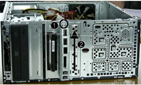
Figure 2-43 Removing the front I/O assembly
